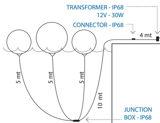
**!** The connector and the transformer must be kept away from water!
