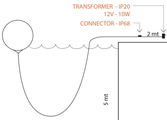
**!** The connector and the transformer must be kept away from water!
